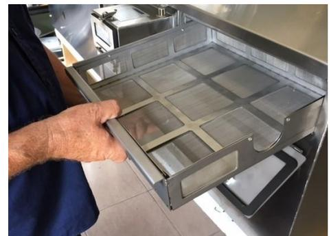
Check your filter basket at least twice daily for the first 2 or 3 days to see how quickly it fills with solids. *Keeping the level of solids down means you will prevent these spilling over into the tank.*
