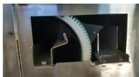
The external wiper may need cleaning daily or weekly, depending on how much solid build up there is. As with the filter, check a few times each day for the first few days of operation to assess how much build up occurs and use this as a guide to how frequently you will need to clean the wiper. When you replace the wiper back in the unit – check to make sure it is back in the correct position. (The edge of the wiper should be resting on the roller)
